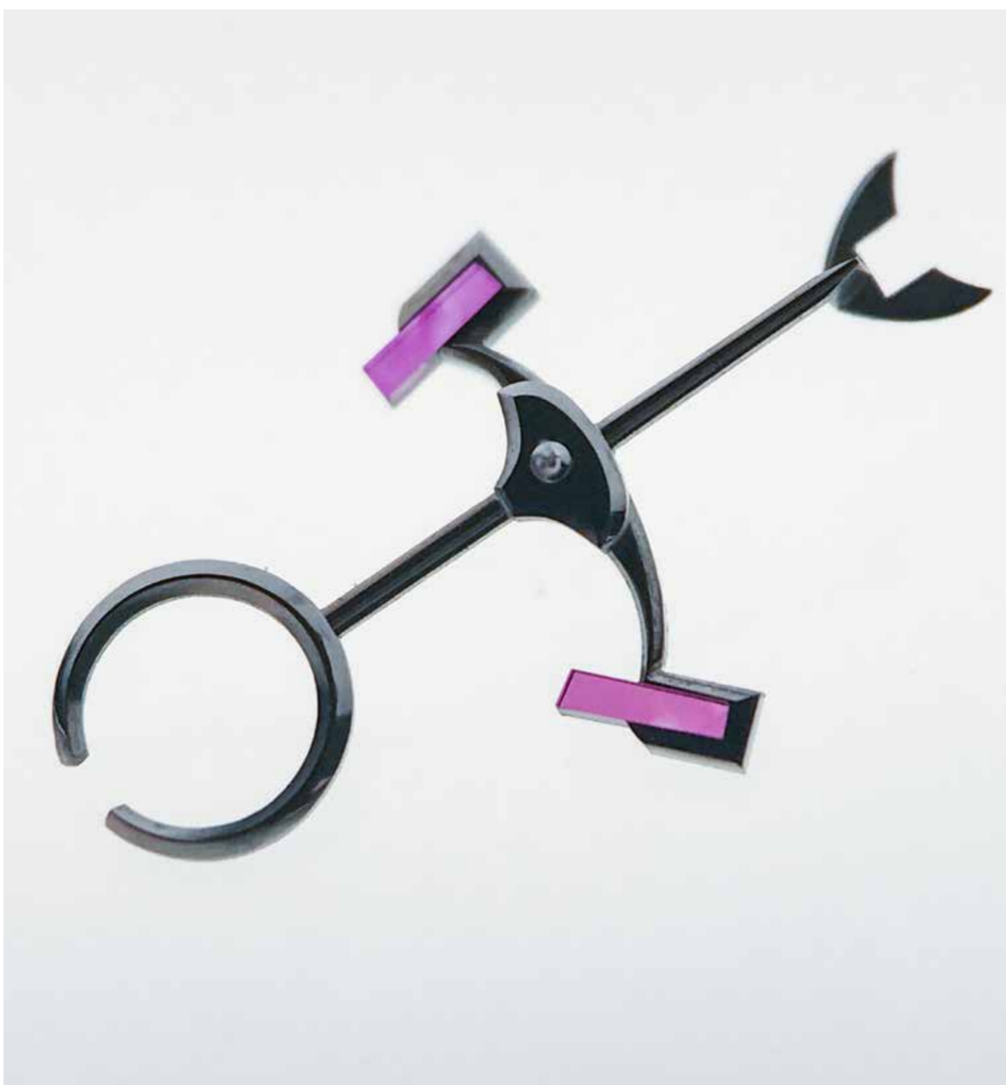
The Swiss lever with counterpoise weight. The cut out in the circle allows the escape wheel axle to pass through during assembly. There is no adjustment possible in the pallet jewels.
